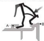
Fig 1 Insert back leading leg into the bead retention slot
