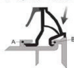
Fig 2 Push downwards or tap with rubber mallet
