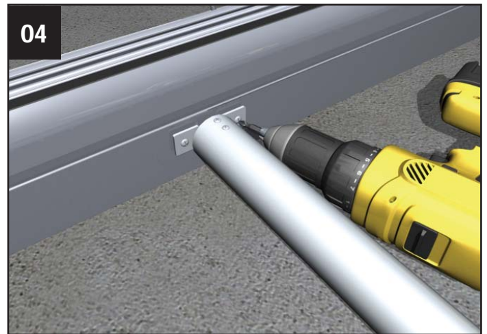
Attach the strut at the mid point of the long sides.
